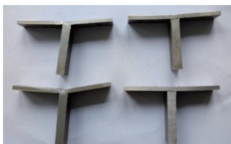
(a) 搭接间隙 0.2 mm
